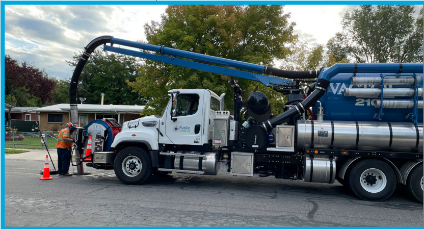
Sewer crews utilize the Department's new Vactor Water Recycler to perform regular cleaning and maintenance
